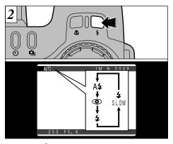
Press the "\$" button to select the flash setting. The flash setting changes each time you press the "\$" button.
